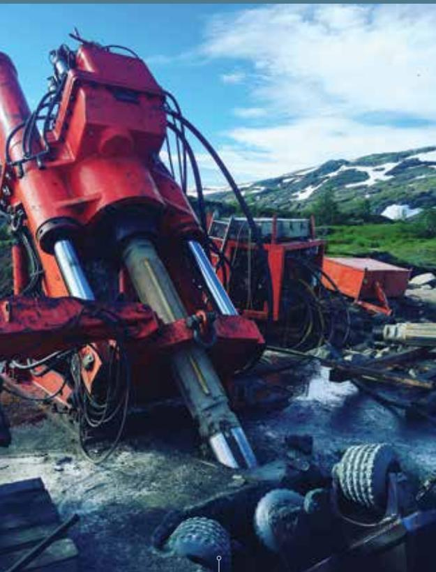
Reamer breaking through top soil after successful diagonal reaming cycle
