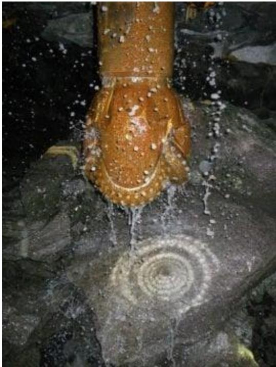
Number 3 shaft currently being developed by Master Drilling through raise-boring, is considered to be safer, quicker and more cost effective than traditional blind-sinking. Raise-boring comprises two key phases: the drilling of a pilot hole, followed by reaming of this hole to its
